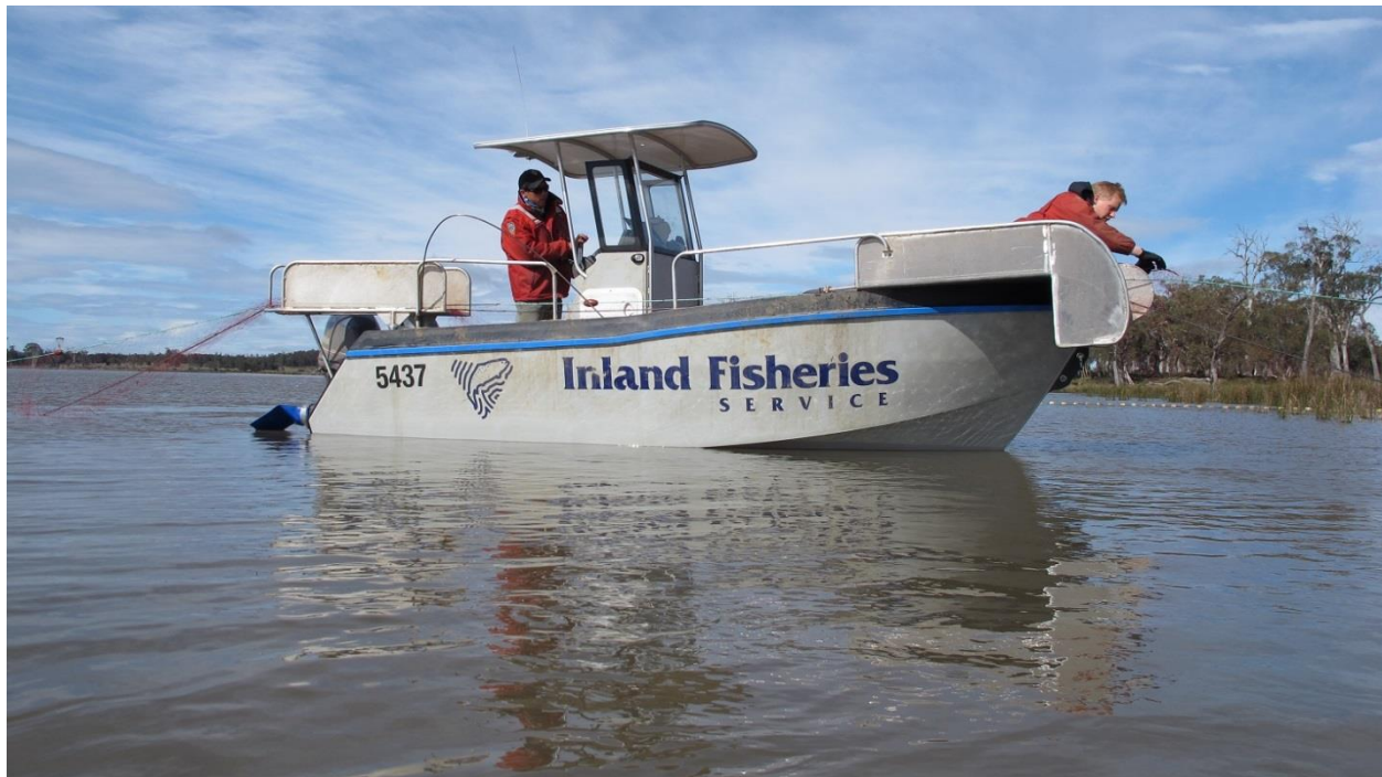
Figure 2. The work vessel IFS10 with the modified net chutes specifically designed for servicing long stretches of gill net
