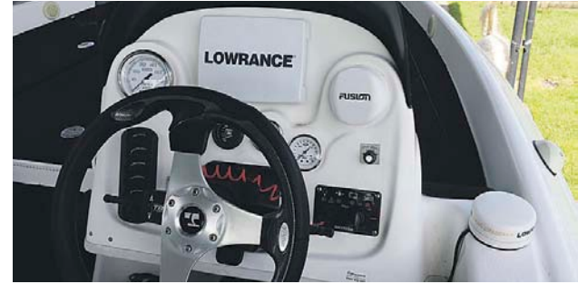
Helm control for trim, tilt and hydraulic jacking plate. Hotfoot throttle.
